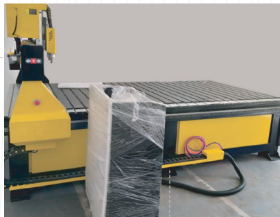
6 Leg body Structure for Stable and reduce vibration
